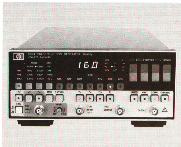
Fig. 1. Model 8116A Pulse/Function Generator has standard function generator capabilities and a pulse mode suitable for testing CMOS and TTL logic. It is HP-IB programmable and operates over a frequency range of 1 mHz to 50 MHz. Logarithmic sweep is optional.
