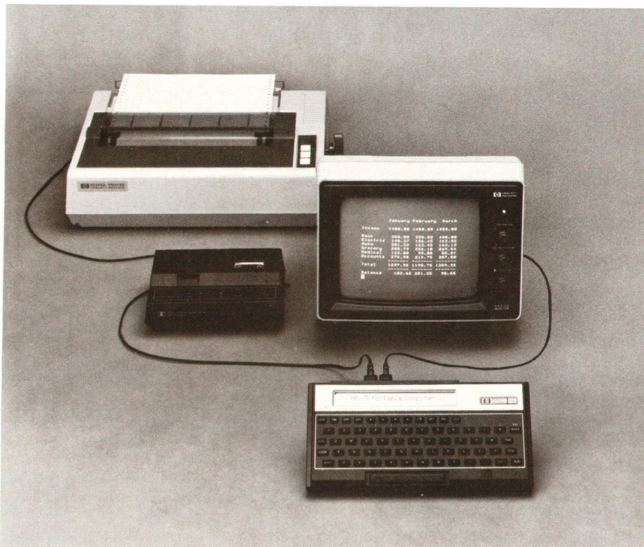
Fig. 2. This HP-75 system features HP's 82168A Acoustic Modem, 82162A Thermal Printer/Plotter, and 82161A Digital Cassette Drive.
