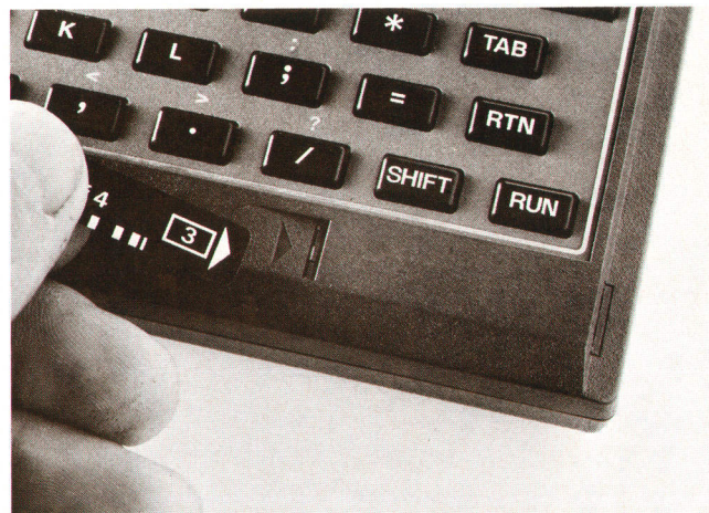
Fig. 1. The HP-75 Portable Computer's internal mass storage system uses a handpulled magnetic card reader and recorder. This unit is located in the lower right corner of the HP-75. Each card can store up to 1300 bytes of data.
