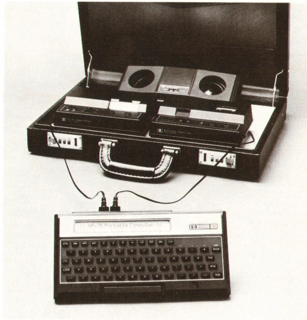
Fig. 2. This HP-75 system features HP's 82168A Acoustic Modem, 82162A Thermal Printer/Plotter, and 82161A Digital Cassette Drive.
